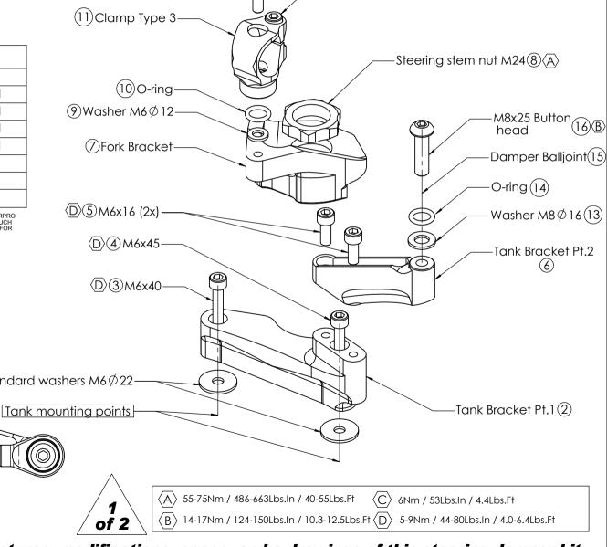
See WWW.HYPERPRO.COM for the latest pictures, modifications, specs. and e-drawings of this steering damper kit.
