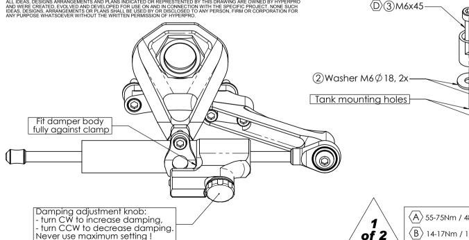
Clamp bolt  $(16)\langle C \rangle$ (10)Clamp Original M24 nut (A) (9)O-ring-(8) M6 Washer- $M8x25(12)\langle B \rangle$ (7)Fork Bracket Damper (13) (D)(6) M6x16 (2x) O-ring(14) M8 Washers (15)  $\langle \overline{D} \rangle (4) M6x50$ -Tank Bracket Pt.2(5) Tank Bracket Pt.1(1)
